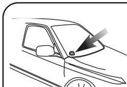
LED light should be installed on the dash board.
